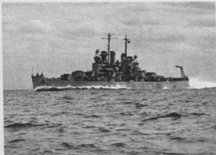
Symmetrical profile of Cleveland's closely spaced stacks, prominent superstructure elements and pole masts show in foreshortened view.
